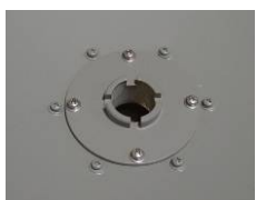
Remove Center Dish Flange
