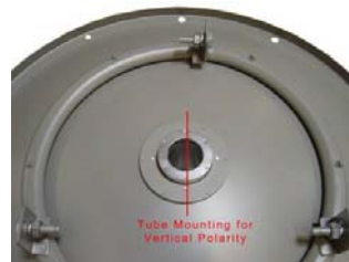
Tube flange orientation for Dual Polarity Feed
