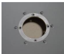
Remove Center Dish Flange
