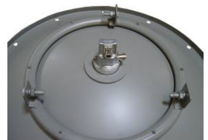
Properly installed Dual Polarity OMT Assy
